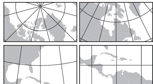
Fig. 8. Landscape format transition between polar Lambert azimuthal (top left), Albers conic (top right and lower left) and Lambert cylindrical projections (lower right) by adjusting standard parallels of the conic.
